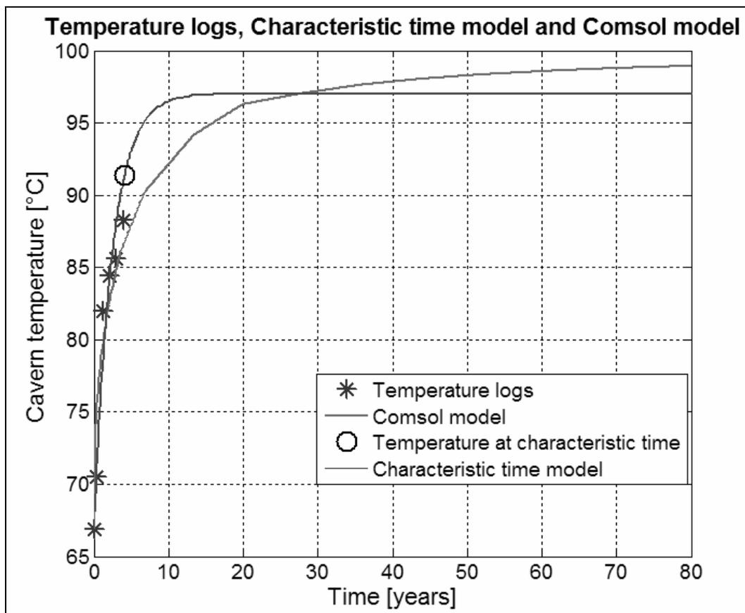
Figure 12. Cavern temperature build-up after shut-in simulations (long term)
