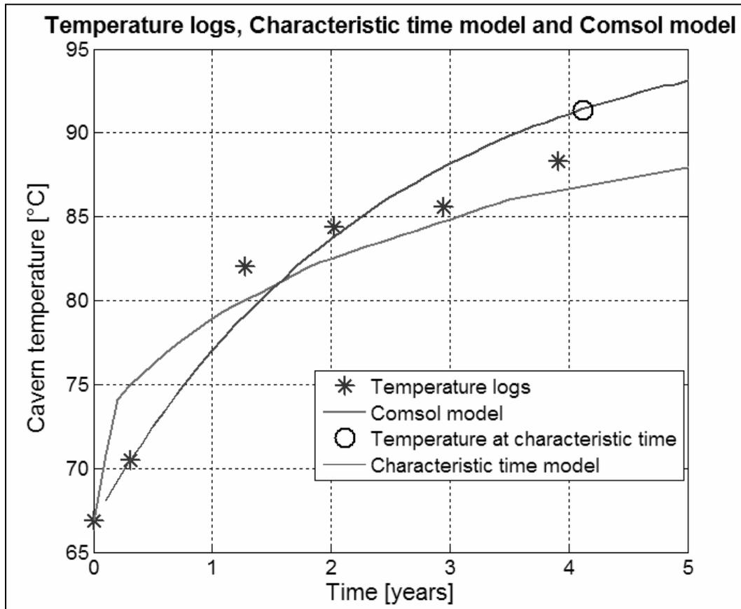
Figure 11. Cavern temperature build-up after shut-in simulations (short term)
